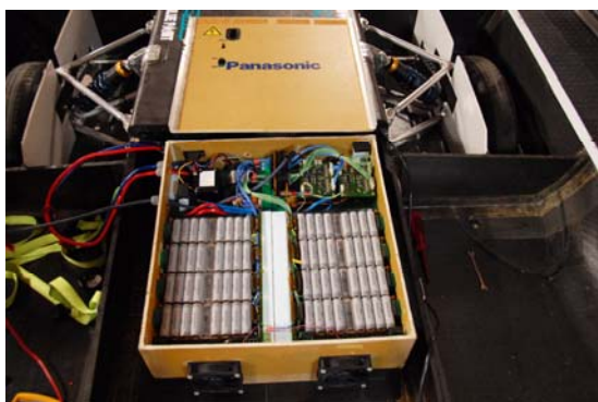
Fig. 4 lithium ion battery.
