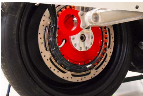
Fig. 3 Brushless DC direct drive motor, carbon disk wheel and low rolling resistance tire.
