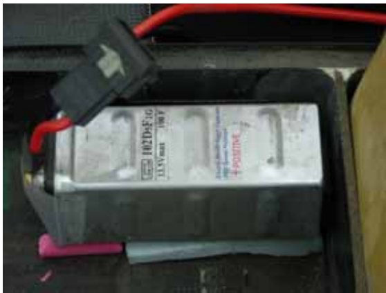
Fig.6 Electric double layer capacitor for the regeneration brake and acceleration.
